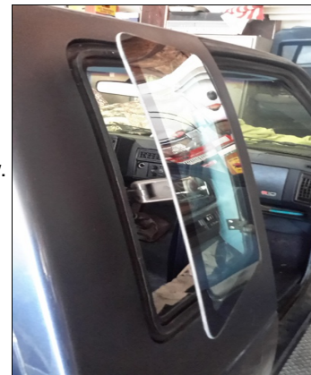
Installed weather seals
